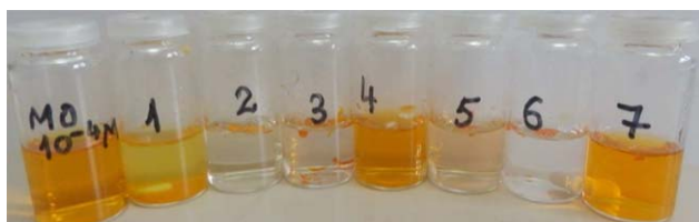
Figure 9. Optical images of the ionic hybrids after the sorption of MO from an aqueous solution with a concentration of 10 -4 M; sorbent dose: 5 mg; volume of dye solution 5 mL; temperature 24 °C; pH ~ 5.5; sample code from the left to the right: (1) S 1 H 2 :1; (2) S 1 H 1 :2; (3) S 2 H 2 :1; (4) S 2 H 1 :2; (5) S 3 H 1 :1; (6) S 3 H 2 :1; (7) S 3 H 1 :2. [Color figure can be viewed in the online issue, which is available at wileyonlinelibrary.com .]
